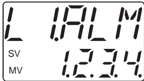
Alarms 1 to 4 are all activated
