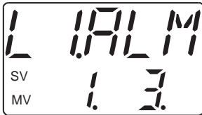
Alarm 1 and 3 are activated
